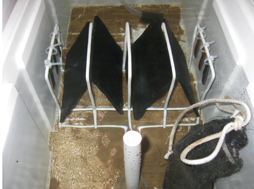
Figure 3. Settlement chamber with settlement plates, corrosion coupons, and mesh bag containing live adult mussels.
