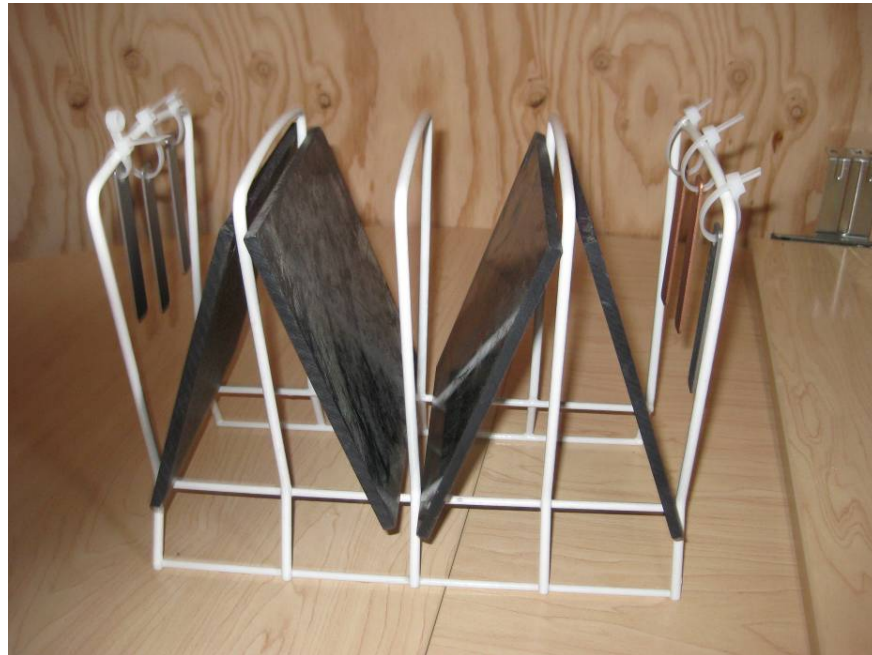
Figure 2. Rack with settling plates and corrosion coupons.
