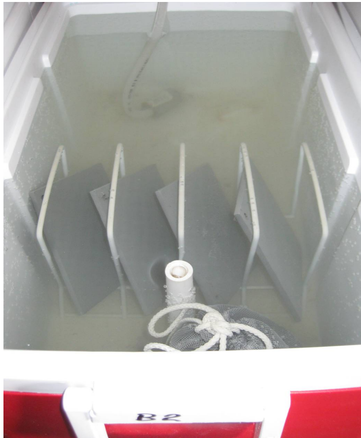
Figure 5. Precipitate observed after 24 hours at pH 9.3.
